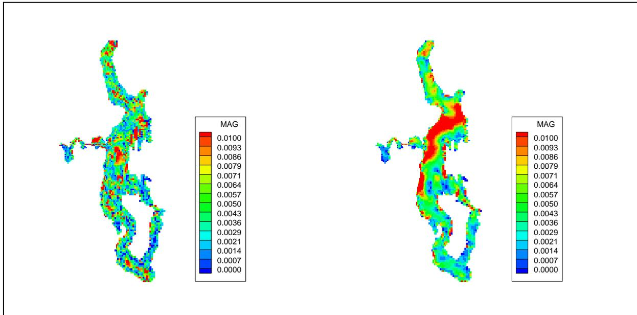
Figure 6. An example time snapshot of the horizontal distributions of velocity magnitude for the bottom layers (Left: SGZ; Right: SIG).
