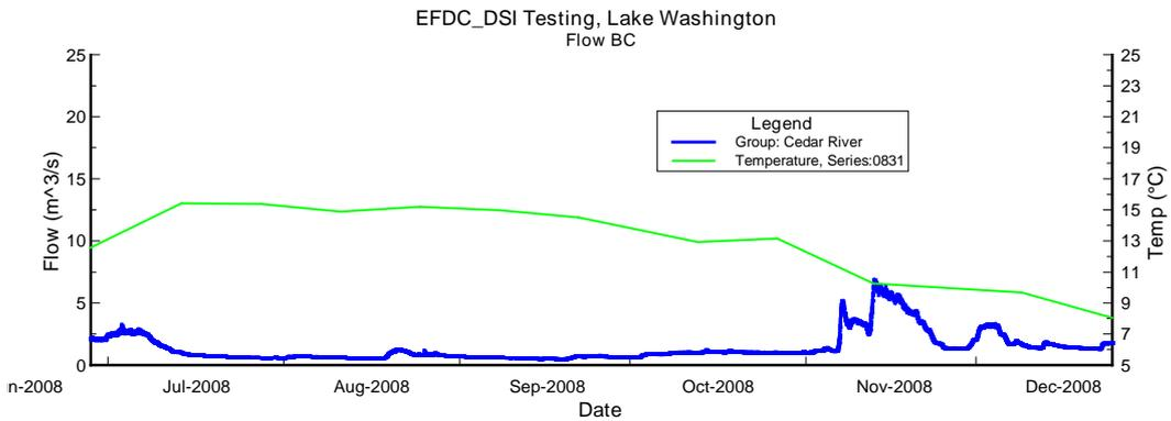
Figure 4. Time series of flow and temperature at Cedar River.
