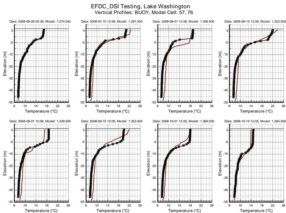
Figure 9. Comparison on vertical profile of temperature between data and computation by SGZ model.
