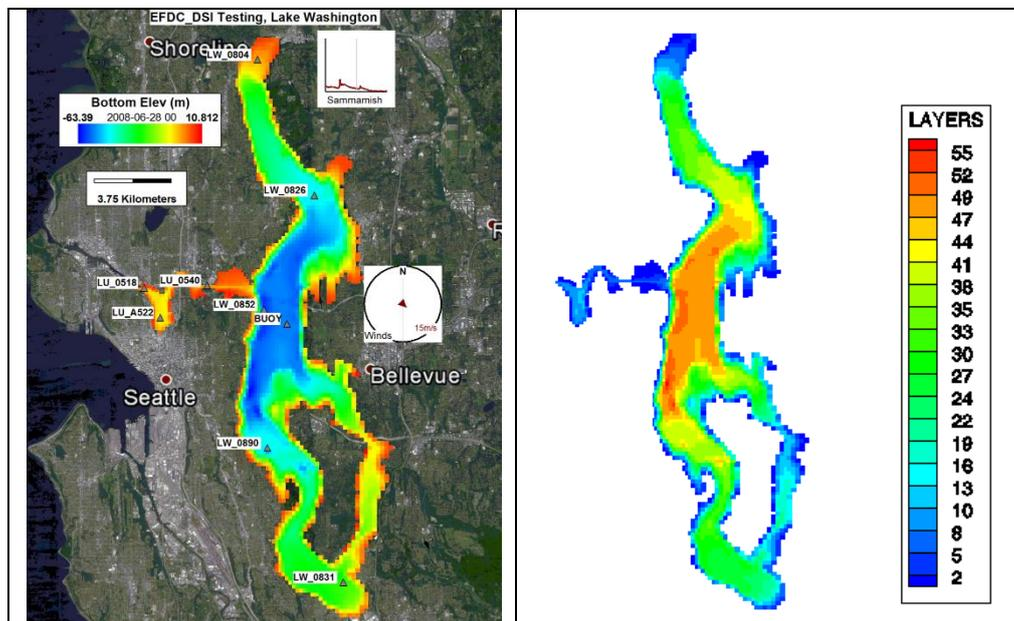
Figure 2. Bathymetry of Lake Washington and number of layers for sigma-zed.
