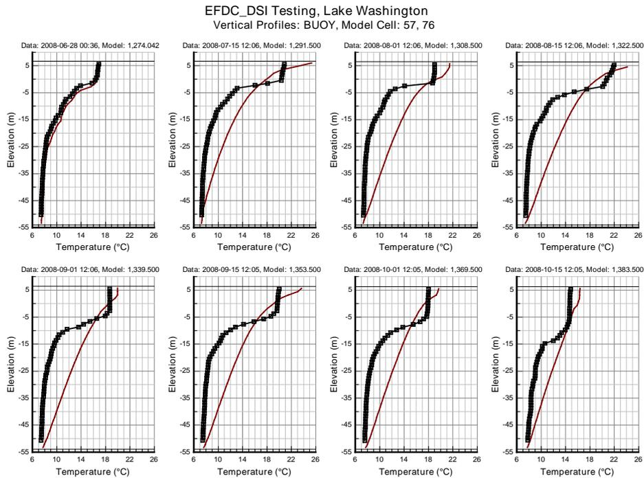
Figure 8. Comparison on vertical profile of temperature between data and computation by SIG model.
