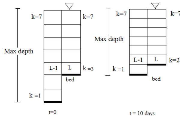
Figure 1. An illustration of SGZ layering before and after a 10 day period with sediment deposition.
